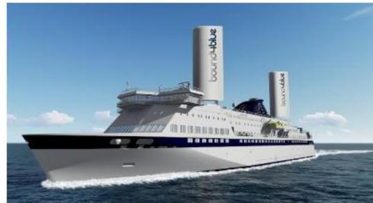
Figure 20 Examples of wind propulsion systems. Extracted from: Díaz, 2020.
