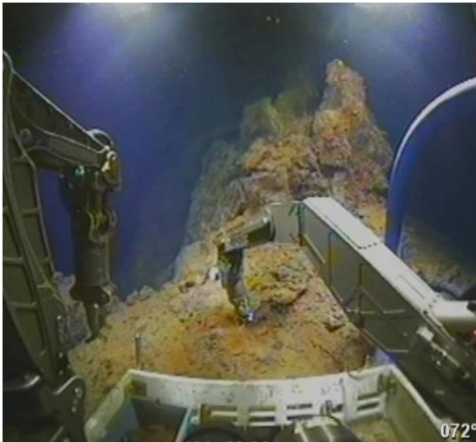
Sampling from sulphide-deposit, 3500 meters water depth in the Norwegian Sea. (Photo: The Norwegian Petroleum Directorate)
